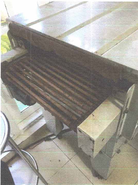
Rust observed in shrink tunnel
